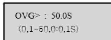
Fig 28) OVGR > Tm(Time Multiply)setup 目錄
